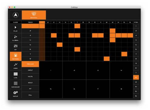
This page shows you the current sequencer grid and allows you to enable/disable steps. You can switch between currently selected track using the menu on the far left. You can clear a row by pressing and holding on a row. Holding for longer will delete all rows.
