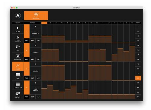
This page gives you access to the 4 parameter animation tracks. Tracks can be enabled/ disabled with the parameter track number button on the far left and armed with the REC button below the track number button.
